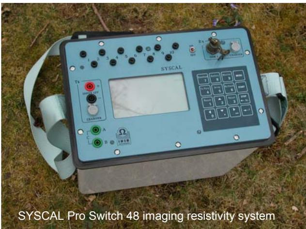
SYSCAL Pro Switch 48 imaging resistivity system
